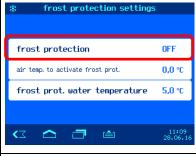
If there is no air temperature sensor connected to the EUROMATIK, these functions are disabled and greyed out.
